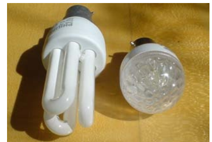
Figure 9.4. Philips 11 W alongside Omicron 1.3 W LED bulb.
