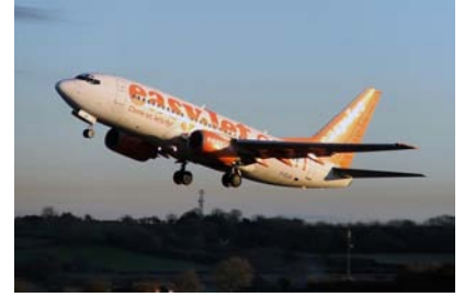
Figure C.11. Boeing 737-700: 30 kWh per 100 passenger-km. Photograph © Tom Collins.
