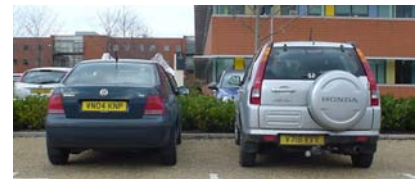
Figure A.5. Power consumed by a car is proportional to its cross-sectional area, during motorway driving, and to its mass, during town driving. Guess which gets better mileage – the VW on the left, or the spaceship?
