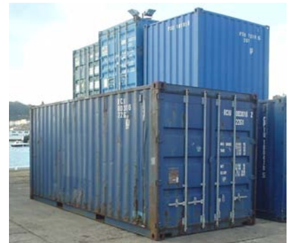
Figure I.4. A twenty-foot container (1 TEU).
