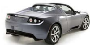
Figure 20.22. Tesla Roadster: 15 kWh per 100 km . www.teslamotors.com .
