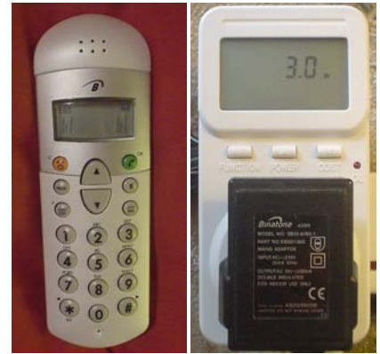
Figure 11.3. This wasteful cordless phone and its charger use 3 W when left plugged in. That’s 0.07 kWh/d. If electricity costs 10p per kWh then a 3 W trickle costs £3 per year.
